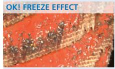
Typical wear pattern with its characteristically shiny cooling film (not glazing!).
