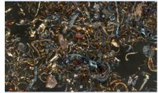
Chips produced with conventional grinding wheels or flap discs. Blue colouration due to overheating.
