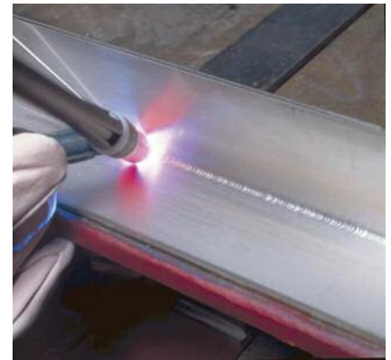
Gas tungsten arc welding on aluminum using ARCAL 1 high-purity argon prevents fusion defects, porosity and weld metal embrittlement.
