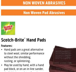
Available in a variety of grades, including aluminum oxide, nepheline syenite, or silicon carbide abrasive materials.
