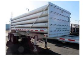
If a higher pressure Nitrogen requirement is necessary, CWS offers Nitrogen trailers capable of holding 40,000 & 50,000CF of Nitrogen at a storage capacity of 2,400 PSIG, and 60,000CF at 2,800PSIG. These units can be delivered directly to the job site for your tank inerting, pipeline purging, pressurization and pigging requirements.
